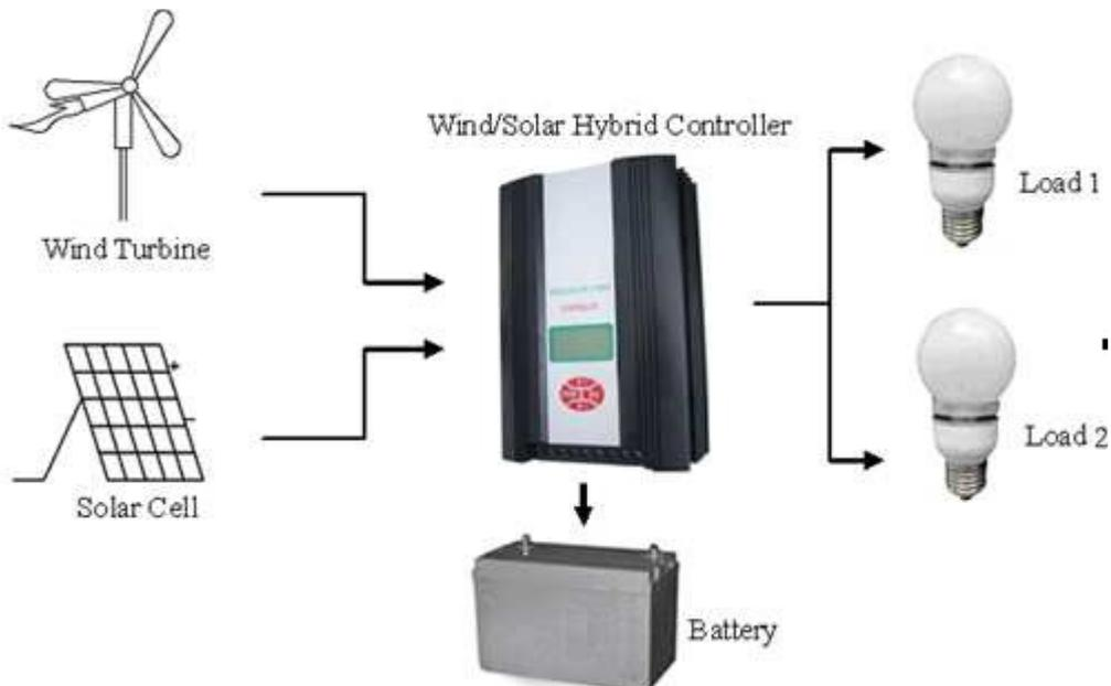
Picture 1, wind&solar hybrid system wiring diagram
